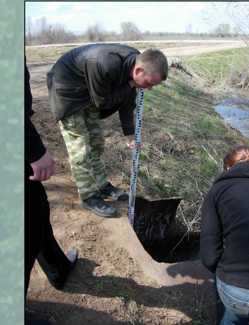
Height and width measurement of culvert
