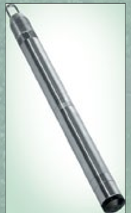
Water level measured with the use of water pressure loggers
