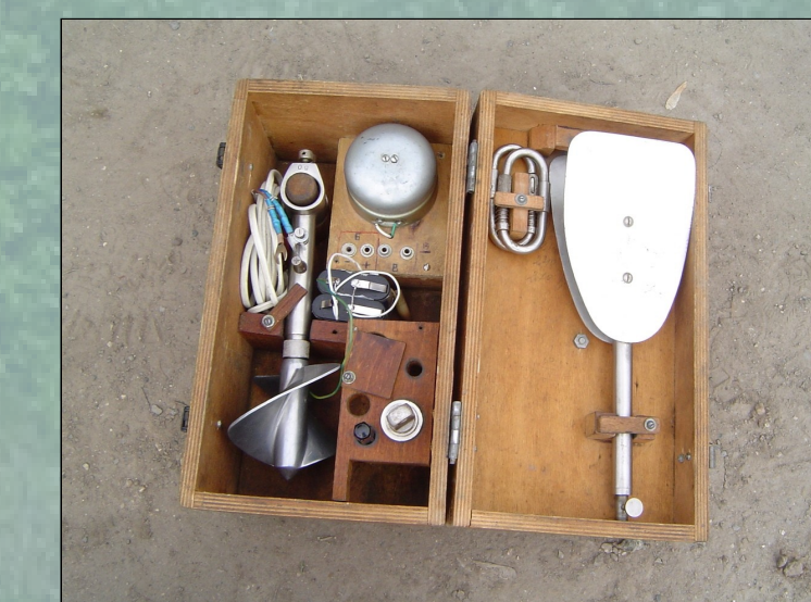
Flow velocity measurement instrument: Ottmill
