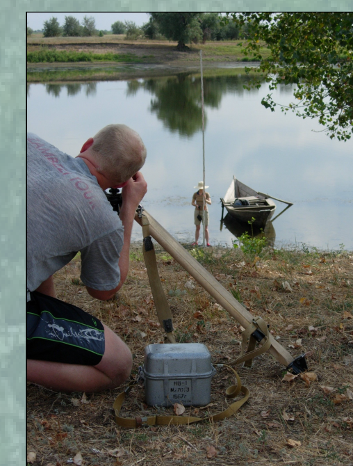
Channel profile measured with leveller
