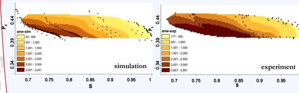
Spatial distribution of interfacial area ( $a_{nw}$ ) within the  $P_c$ - $S$  loop: a) simulation b) experiment
