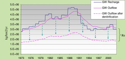
Nutrients leaching to the groundwater store are retained based on the residence time before entering surface water. Part is denitrified during transport.
