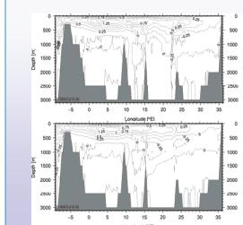
Annual mean zonal overturning stream function. Upper panel: Reference experiment. Contour interval is 0.25 Sv. Lower panel: as previous for experiment with Nile discharge adjusted to 5 times the precession minimum value.
