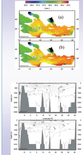
MOMA Sea surface salinity in February (average of years 15–20). (a) Reference experiment, (b) experiment with Nile discharge adjusted to 5 times the precession minimum value.
