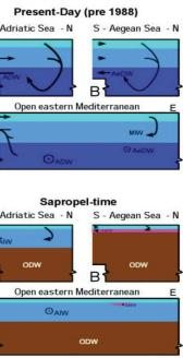
Schematic presentation of hypothesis of the changes in subsurface circulation patterns between the present day (upper panel) and times of sapropel formation (lower panel) [Rohling, 2001].
