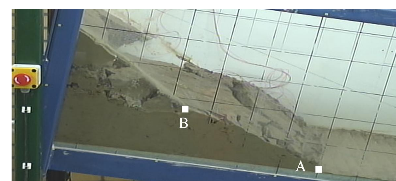
Fig. 10: Slope after failure, 26-10-2008, inclusive final positions of observed points A, B.
