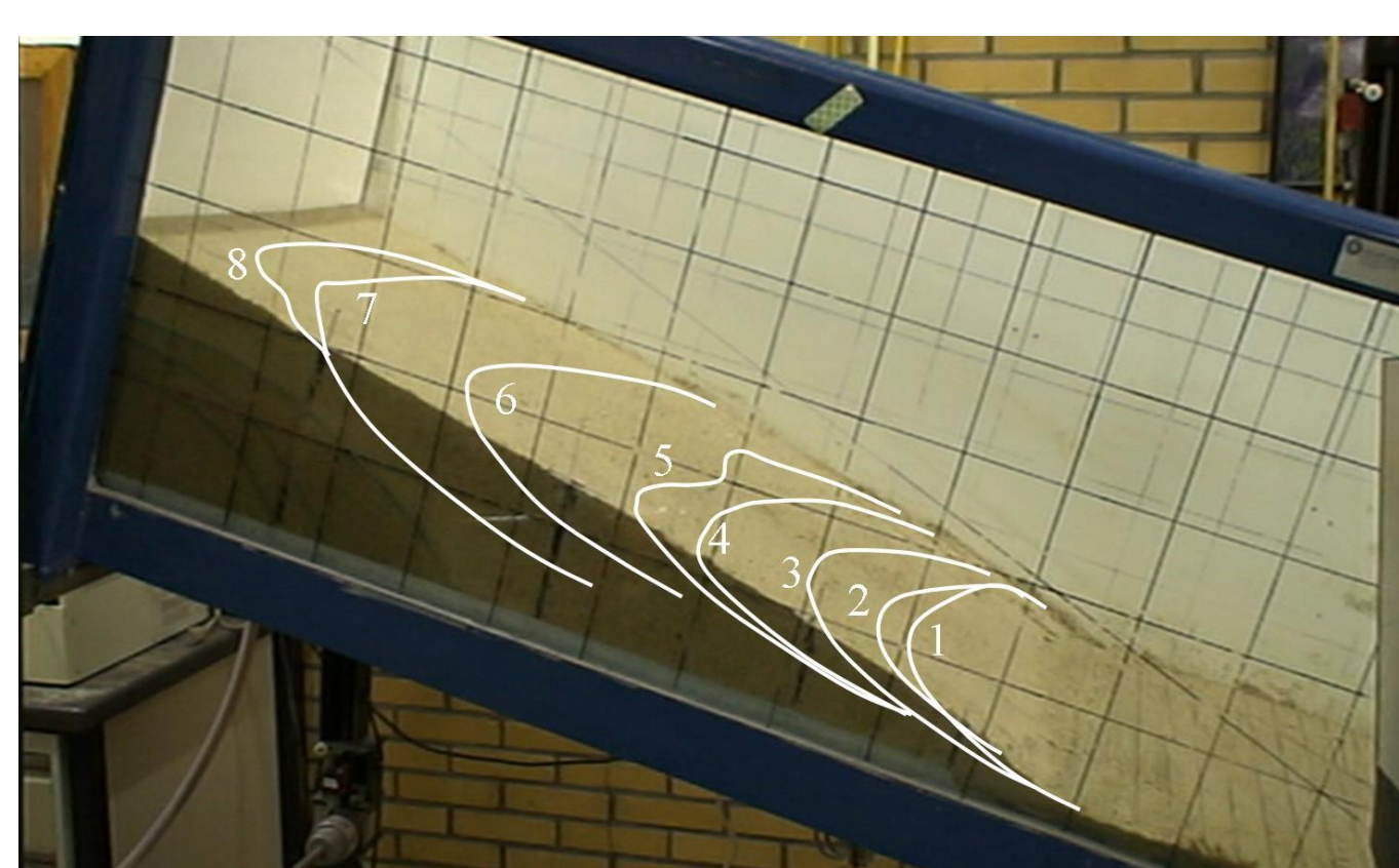
Fig. 5: Geometry and sequence of slumps during retrogressive failure.
