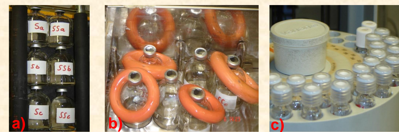
Fig. 1: Completely mixed batches at a) room and b) 30 °C temperatures with c) measuring vials positioned in an auto-sampler.
