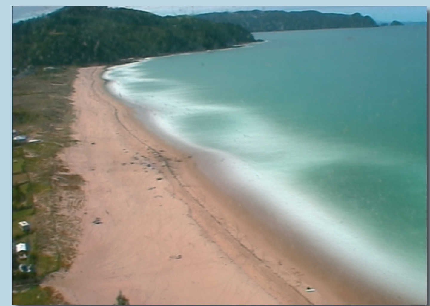
Figure 2. Applied video imagery technique showing Cam-era time-exposure image.
