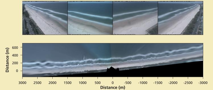
Figure 2: The four oblique, 10-min time-exposure images are merged and rectified to yield a plan view image. The two alongshore white lines represent wave breaking on the sandbars.
