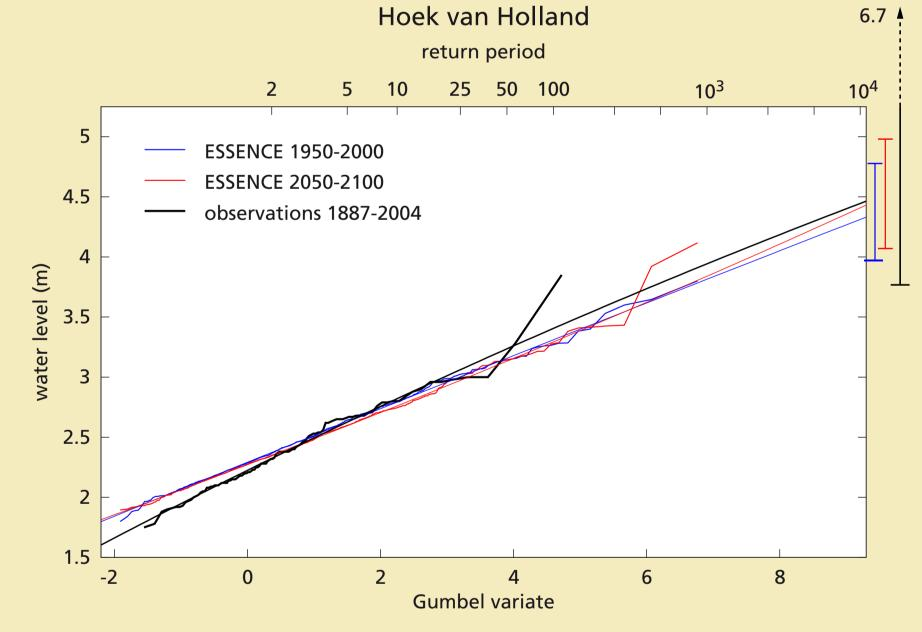
Gumbel plot for water levels at Hoek van Holland from the ESSENCE-WAQUA/DCSM98 ensemble. Black: observations, blue: present-day climate (1950-2000), red: future climate (2050-2100). The thin lines are the fits to a GEV, and the bars in the right margin indicate the 95% confidence interval of the 10 000-year return value. Within the limits of natural variability there is no change in the height of the water levels due to global warming along the Dutch coast. [Sterl et al 2009]
