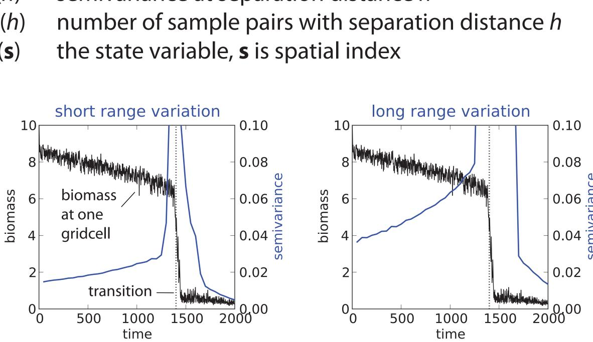
The panels above show a marked increase in semivariance, representing short distance (left) and large distance variation (right). Thus, an increase in spatio-temporal variation in biomass can serve as warning signal for degradation of the soil at 1400 years.
