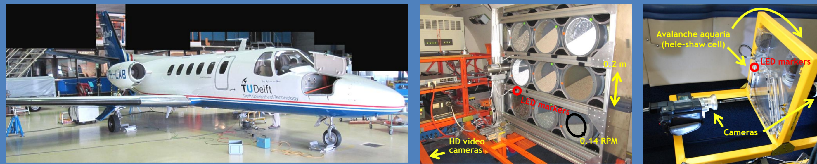
Figure 3.1 Our flying laboratory aircraft: the Cessna Citation II (left), the rotating drum set-up to test various sediments and interstitial media (centre) and the hele-shaw cells.
