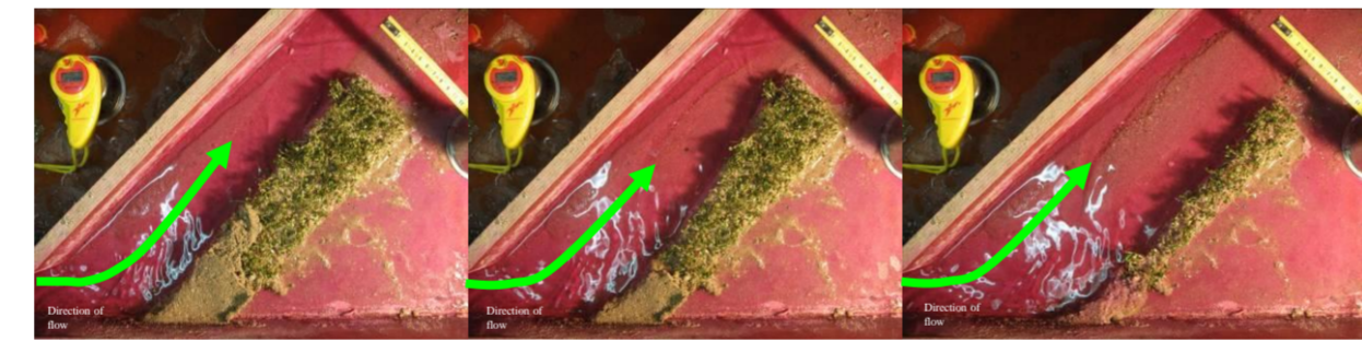
Friedkin experimental setup showing the erosion of a block of sediment with a high density of rucola sprouts after 0, 40 and 70 minutes.
