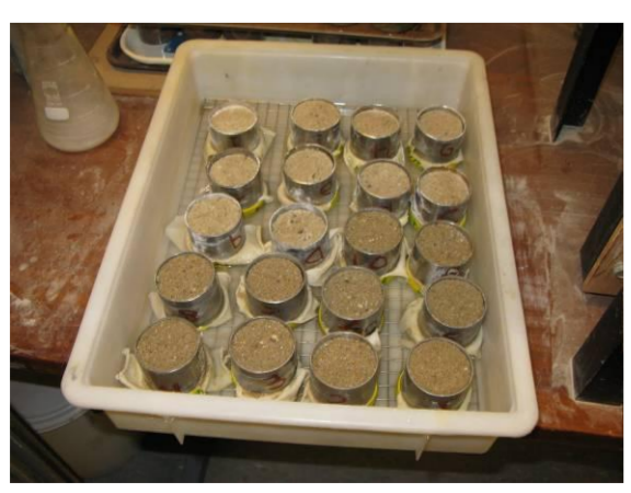
pF-curve samples (fixed volume of 100 ml) of poorly sorted sand and a sand-silica flour mixture. Samples are bathed before they are saturated.
