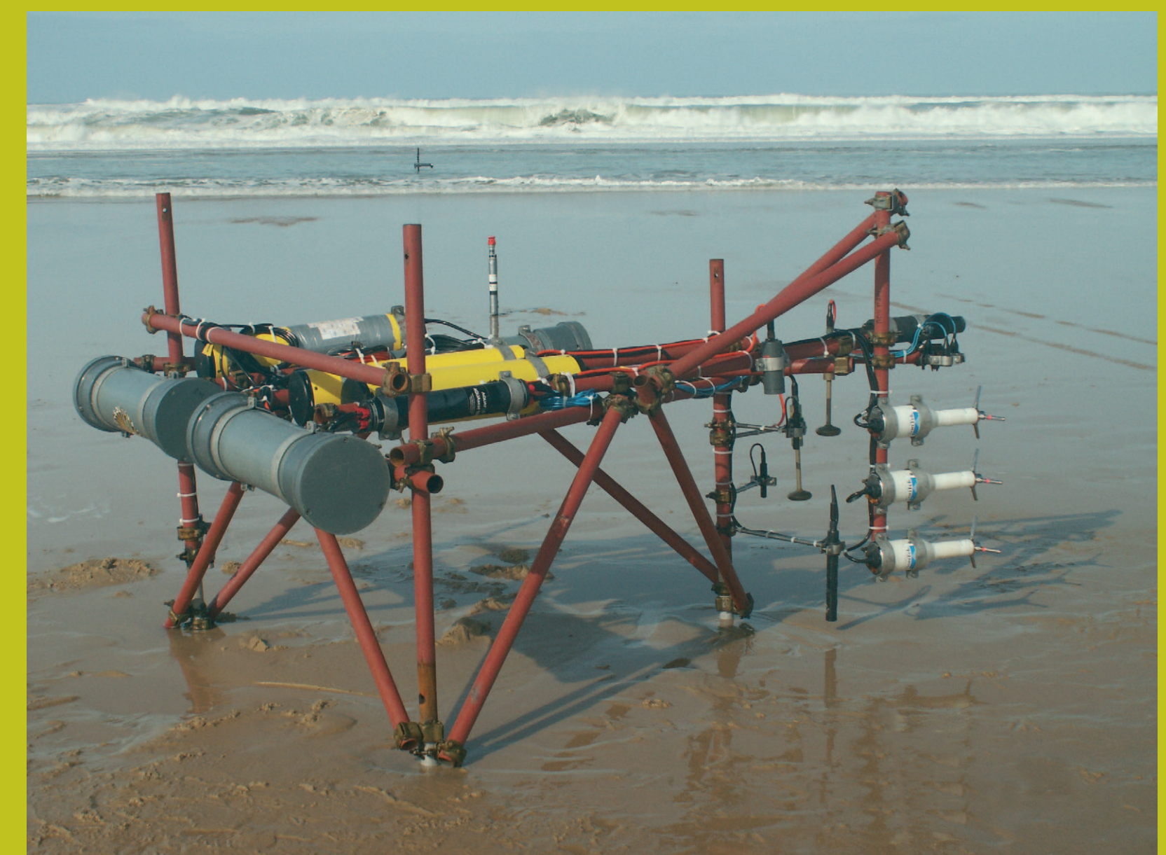
Figure 2. Instrumented rig at low tide. Wave velocities are measured by three ADVs during high tides.
