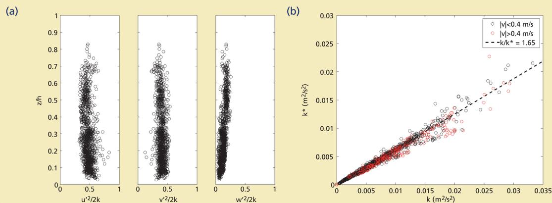
Figure 3: (a) Relative contribution of  $u'^2$ ,  $v'^2$  and  $w'^2$  to  $2k$ , plotted against normalized instrument height  $z/h$ . (b)  $k$  against  $k^*$ .
