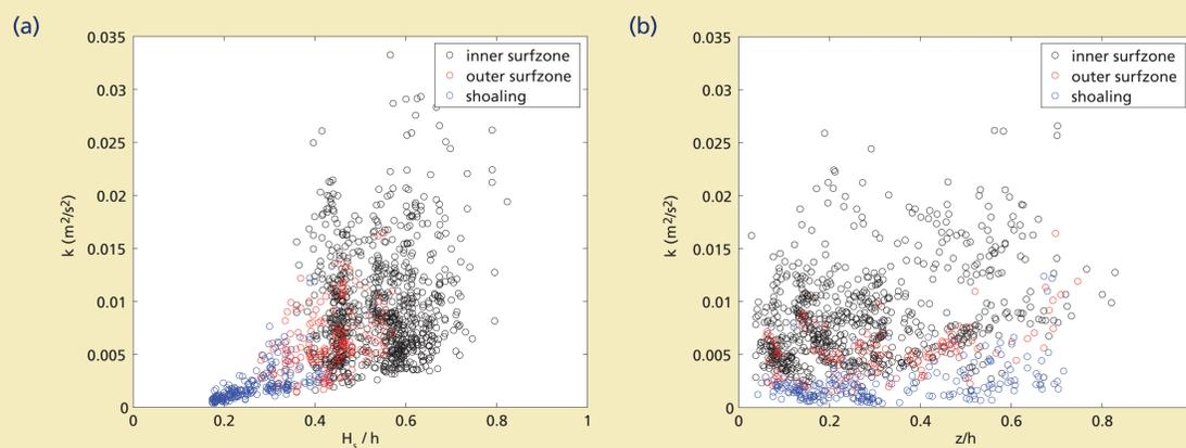
Figure 2: (a)  $k$  against  $H_s/h$  for inner/outer surf zone and shoaling waves, (b)  $k$  against  $z/h$  for inner/outer surf zone and shoaling waves.  $z/h$  is the relative position of an ADV,  $z/h = 0$  is the sea bed, and  $z/h \approx 0.7$  is the wave trough level.
