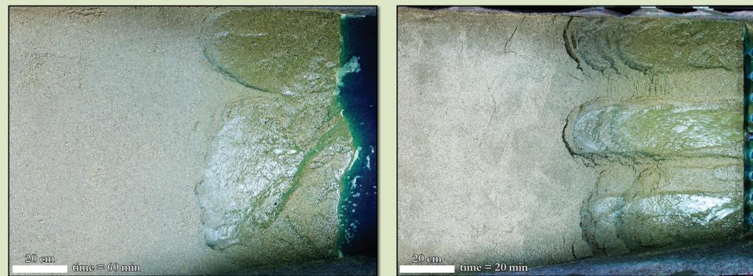
Fig 5) Sapping experiments in wide flume. In the experiment in the left panel, eroded material is allowed to deposit, in the experiment shown in the right hand side panel, sediment is flushed out of the system. In the experiment with deposition, channels became much wider than the channels where the sediment was removed downstream. Also the latter developed much quicker.
