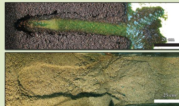
Fig 4) Sapping experiments in narrow flume (also see Kleinhans 2010). Sapping channels form when eroded material is transported sufficiently but headward erosion stops when the channel gets 'blocked' by its own deposits.
