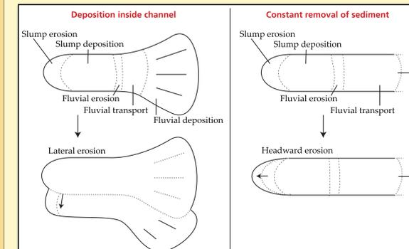
Fig 6) Deposition of sediment causes the sapping channel to widen as the channel head is no longer destabilized and downstream avulsions trigger lateral migration of the channel. Removal of sediment is required for the sapping channel to develop in headward direction.
