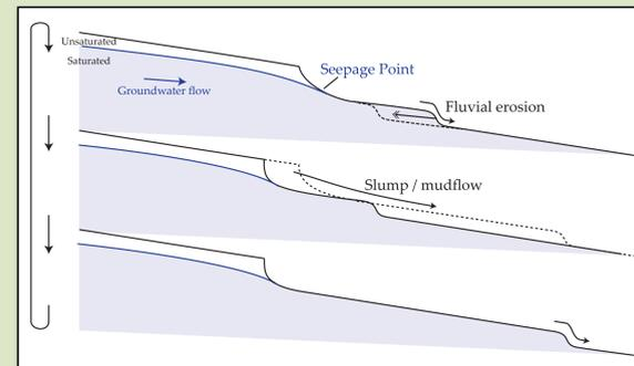
Fig 3) Processes observed in sapping groundwater experiments: mass movements of the head of the channel and fluvial processes further downstream, the latter destabilized the channel head and triggers slumping of the channel head.
