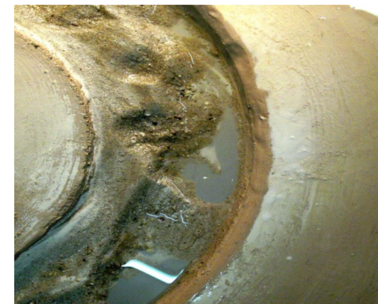
Minimal inundation levels (0,5mm) resulted in silica flour deposition along the channel
