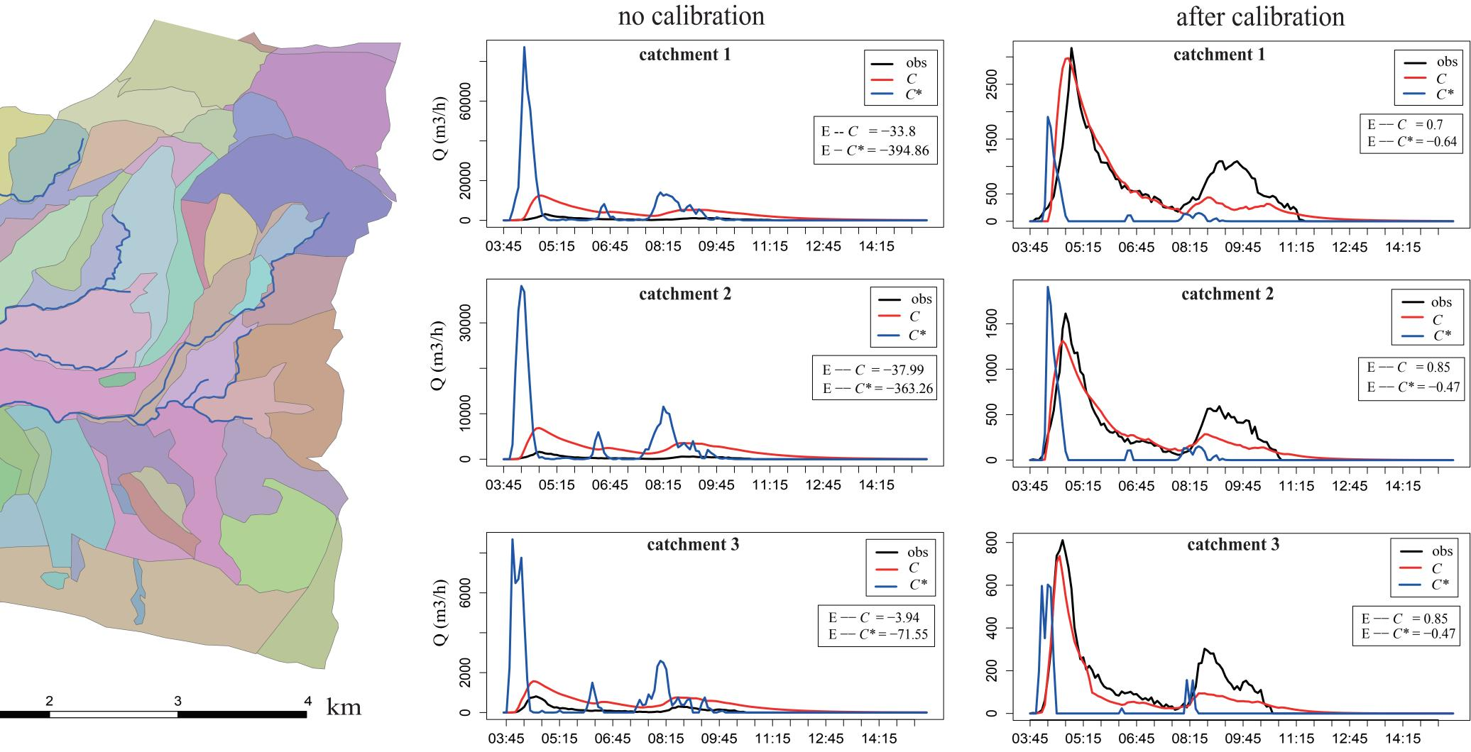
• 15 km<sup>2</sup> catchment in French Alps (3 sub-catchments with total 60 REWs) • 12 rain gauges, 3 discharge gauges, 1 meteostation
