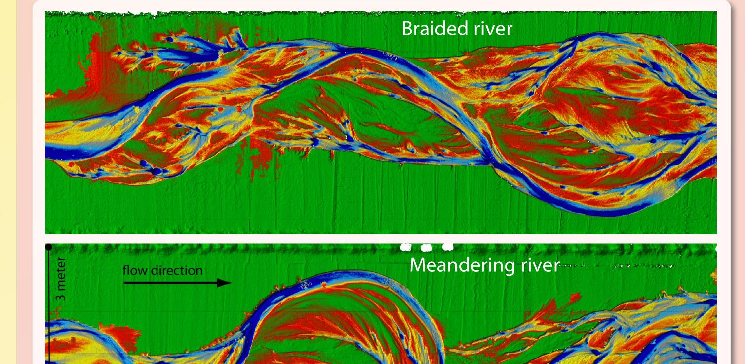
Fig. 6. Detrended Digital Elevation Maps of an experimental braided and meandering river after 120 hours of flow. Both rivers had lateral migration of the channel, but the deposition of silt led to sustaining of the meandering rvier due to less number of chute cutoffs (Van Dijk et al., 2013).
