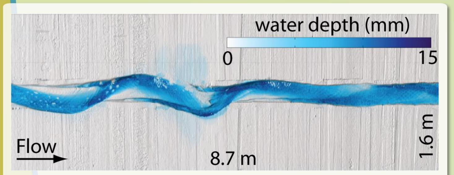
Fig. 3. Shaded Digital Elevation Model with blue colors to indicate the water depth. A series of alternate bars developed from an initial straight channel with a static perturbation, so that alternate bars are formed from upstream to downstream direction.
