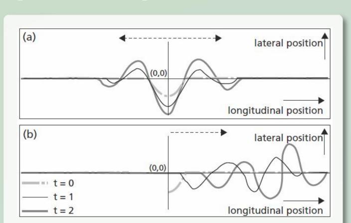
Fig. 2. Migration of a perturbation of the channel planform. (a) Absolute bend instability spreads in both direction. (b) Convective bend instability only migrates in downstream direction in the case of sub-resonant conditions and the dynamics decrease after the perturbation.
