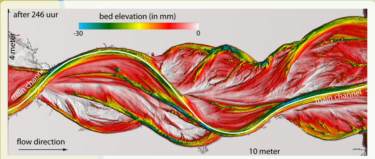
Fig. 4. The continuously transverse moving upstream boundary caused high-amplitude dynamic meandering river with scroll bars and infrequent chute cutoffs. After chute cutoffs, the former channel was closed by a plug bar and new meander bends were formed (Van Dijk et al., 2012).
