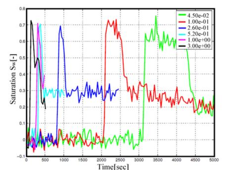
Fig7. Saturation breakthrough curves for different flow rates in cm/min,  $S_{init}=0$
