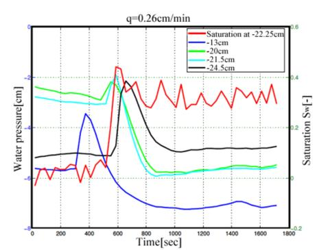
Fig9. Distribution of saturation at one position and pressure at multi-positions
