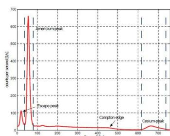
Fig4. Characteristic curve for gamma system
