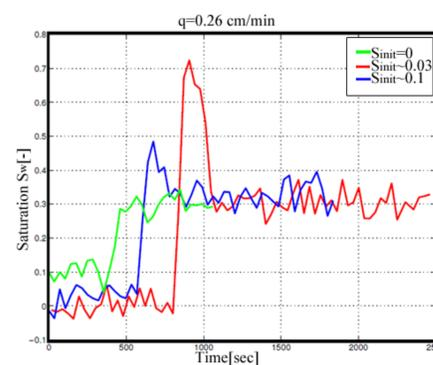
Fig8. Saturation breakthrough curves for different initial water saturation
