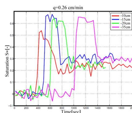
Fig10. Breakthrough curves at different positions with equivalent flow rates
