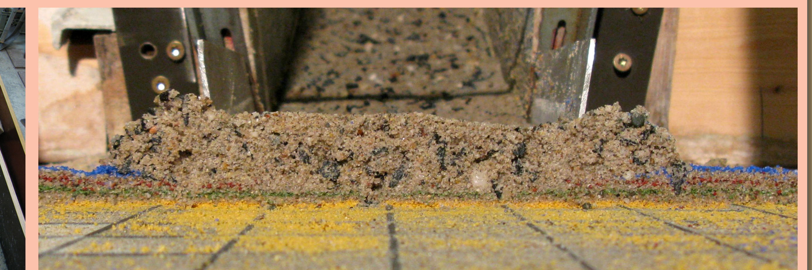
Fig. 10) Debris-flow erosion experiment. We use an initial bed layered with colored sand, in order to determine the erosive depth in the runout zone.
