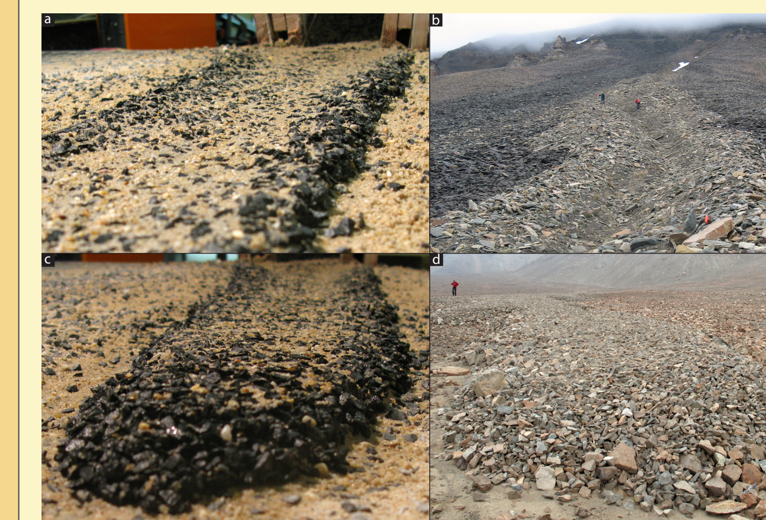
Fig. 7) Comparison between sediment sorting of experimental (a,c) and natural (b,d) debris flows.
