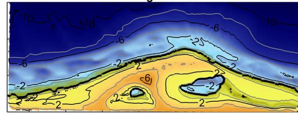
The Sand Engine is expected to be fully incorporated in the beach and dunes within 20-30 years by the action of wind, waves and currents.
