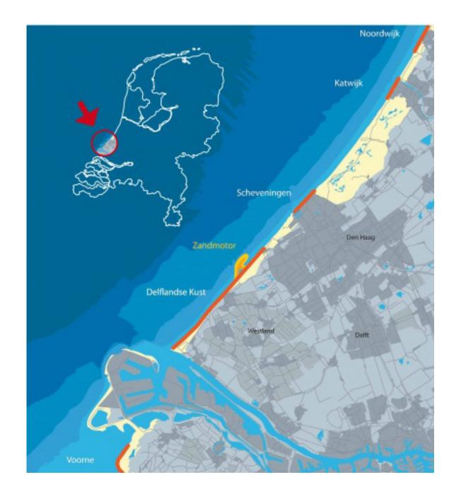
To protect the Dutch hinterland from flooding sand is applied on the coastline since 1990. Because of a rising sea level the coast will become more vulnerable in the future and therefore the Netherlands is in need of a new coastal defence method. The innovative approach of the Sand Engine gears towards sustainability in which coastal defence goes along with ecology and recreation: Building with Nature!
