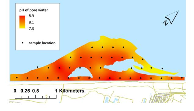
pH of pore water is around 7.5 along the coastline and increases to 8.9 where the unsaturated zone is > 1m thick and freshening occurs.
