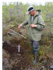
Installing Diver in piezometer In Ryam. Photo: E.Lapshina
