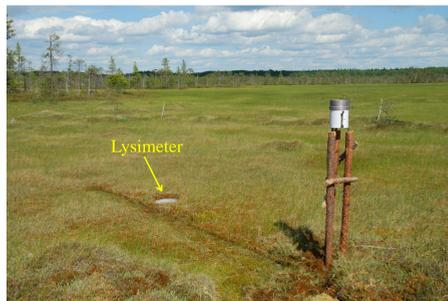
Rain gage and lysimeter for open water evaporation measurement Photo: E.Zarov
