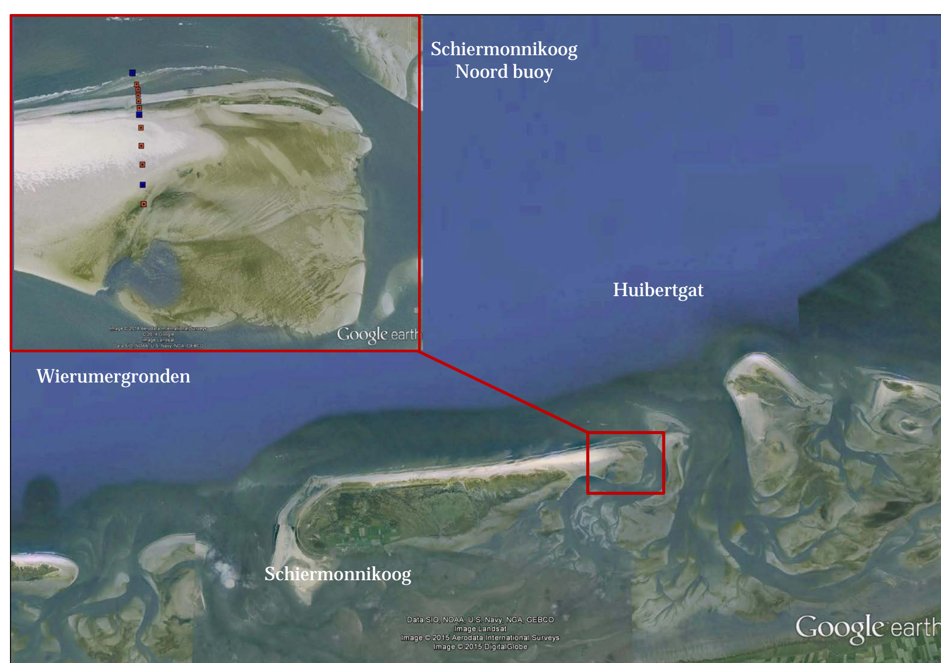
Figure 1. The field site is located on the Dutch barrier island of Schiermonnikoog. Approximate locations for available wave - and water level data (RWS) are indicated. The instrument locations of ADVs (blue squares) and pressure sensors (orange squares) are shown in the inset.
