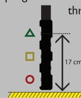
Schematic representation of the lowest five sand concentration sensors between 4 and 17 cm above the bed. Three are used for the analyses here, indicated with a red circle, yellow square and green triangle.
