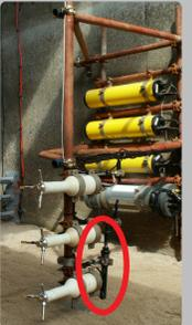
The measurement rig in the flume. The sand concentration instruments are encircled. Turbulence was measured using the three ADVs.
