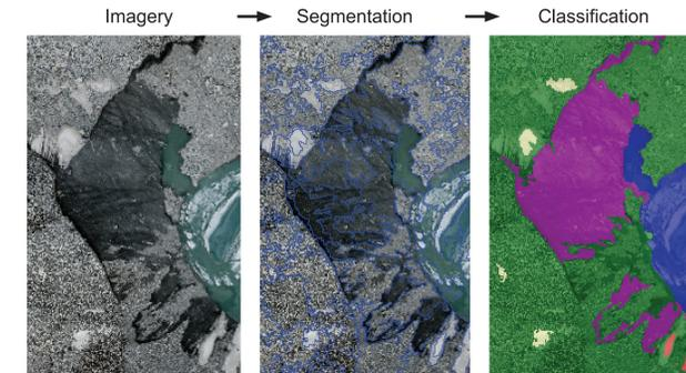
Figure: Basic object-based image classification procedure.
