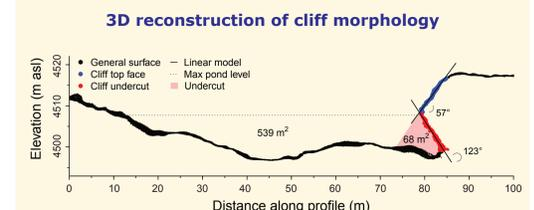
Figure: Cross-section of the UAV-derived point cloud of a cliff. The UAV is capable of capturing undercut morphology because of the low flight altitude and oblique images. Systematic volumetric 3D analyses of multi-temporal point cloud data may provide valuable information about the changes in cliff morphology and their causes.
