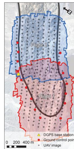
Figure: The coverage of the two UAV flights that were performed on the 7th of May ground control markers and the DGPS base station.
