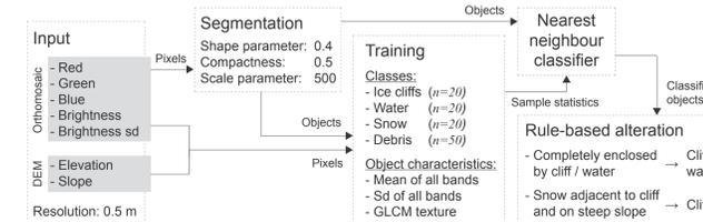
Figure: Flowchart of the steps and settings used in OBIA procedure that was performed to classify the cliffs and ponds from UAV imagery.
