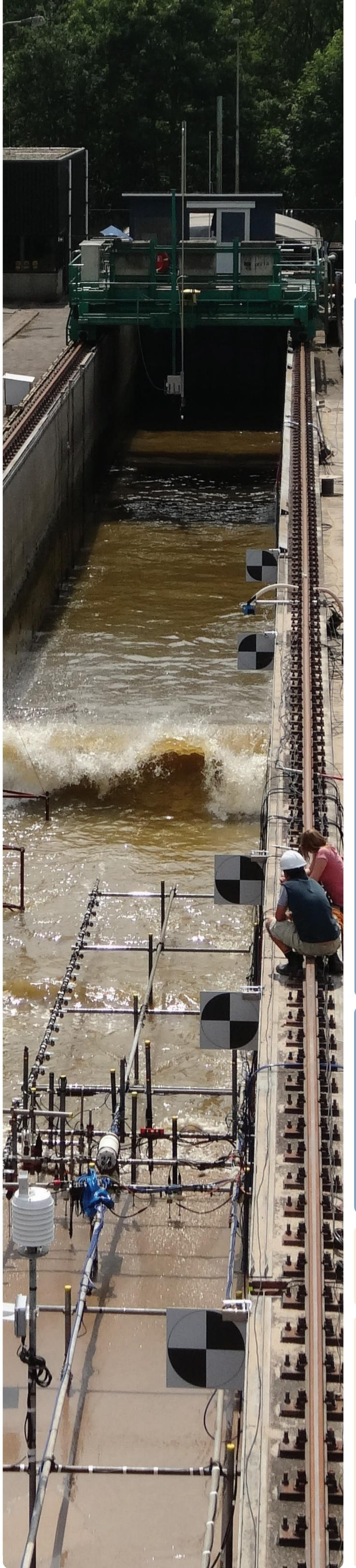
Here, we compare sand stirring by breaking waves to non-breaking waves above ripples by using laboratory measurements collected during the Barrier Dynamic Experiment II (BARDEXII).
