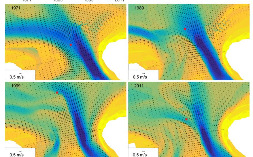
**Figure 4** Vector plot of the residual depth-averaged flow for intermediate, Northwest wave conditions. The center of the residual circulation cell is indicated by a red dot. Bathymetry shown in colors, ranging from -25 m (blue) to 5 m (yellow). Dashed line represents same cross-section in inlet as in Figure 2.
