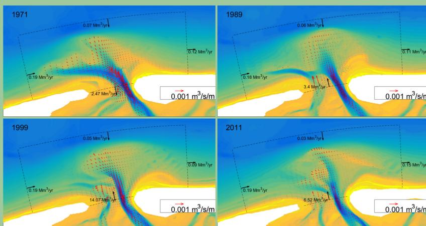
**Figure 2** Weighted mean of total load sediment transport (red vectors). Bathymetry shown in colors, ranging from -25 m (blue) to 5 m (yellow). Dashed lines are cross-sections over which sediment transport over a year is calculated (black arrows and numbers).
