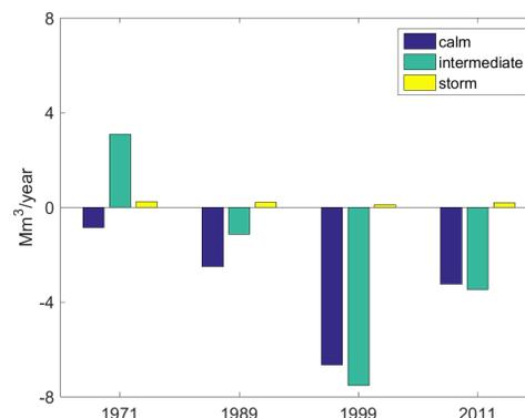
**Figure 3** Bar plot of the sediment import/export for the four historic bathymetries, differentiating between calm weather, intermediate weather and storm. Positive (negative) values indicate import (export).
