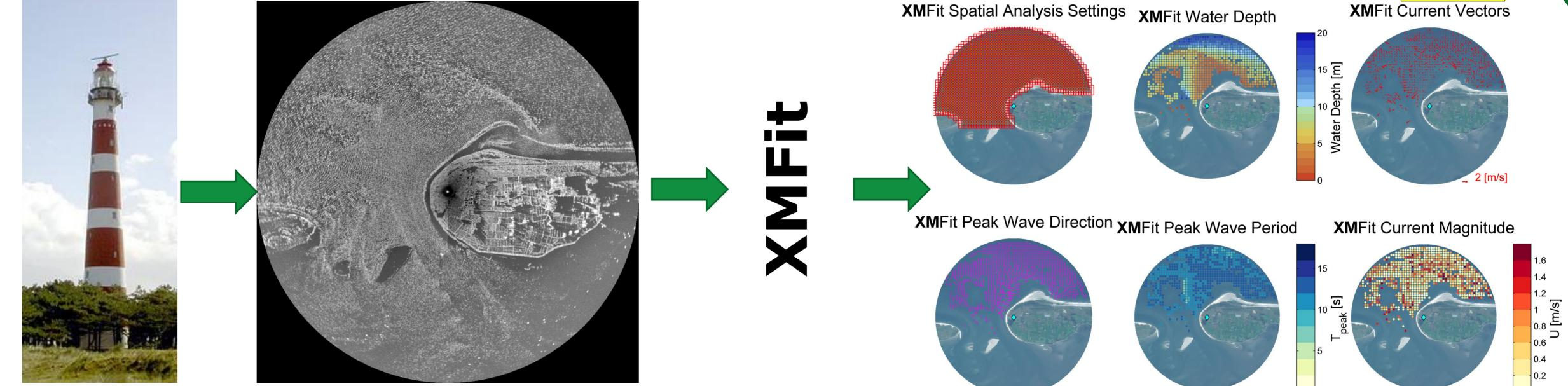
The X-band radar system on the lighthouse of Ameland gives an image of sea clutter every 3 seconds. The XMFit model processes this and returns water depth (bathymetry), current direction and magnitude and peak wave direction and period. Thus, the relation between hydrodynamics and morphodynamics can be studied.
