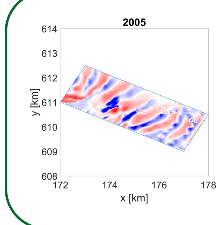
**Left**: the saw-tooth bar field north of Ameland in 2005. Saw-tooth bars are approximately 2m high and have a wavelength of 500-1000m. They are always found on the downstream part of the ebb-tidal delta lobe, in water depths of 5-10m.
