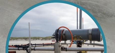
**Small transport rigs,** measurements of pressure (water depth, wave height), horizontal flow velocites and sand concentrations. These rigs are used to understand sand transport gradients over the intertidal zone.
