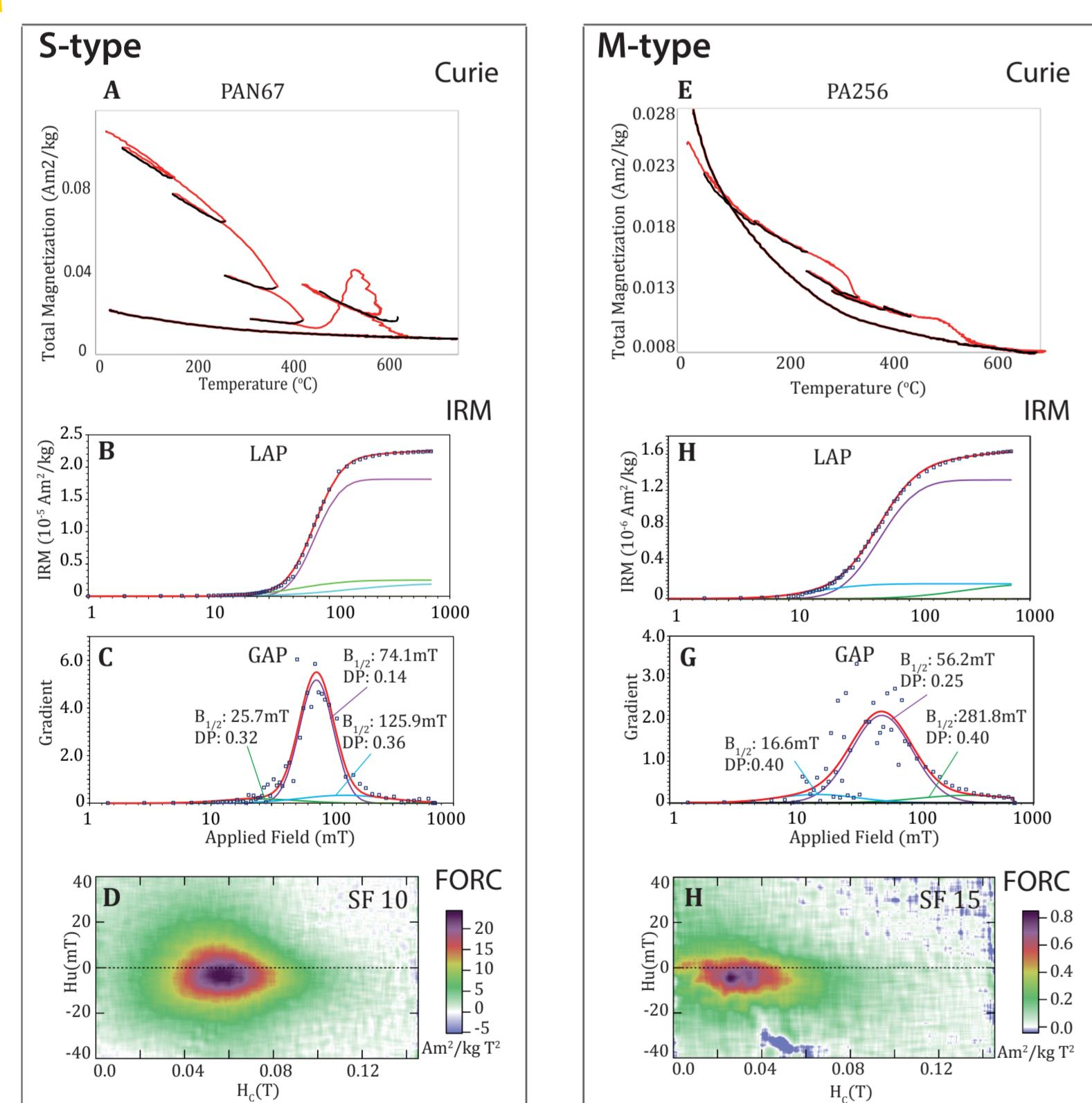
**Left:** A clear greigite sample. A) Irreversible decrease in magnetization ~250–400 °C depicts greigite break-down. Pyrite to magnetite peak between 400 and 580 °C; B/C) IRM values in the greigite range; D) Slightly negative peak at 50–60 mT, closed large concentric contours, indicative of SD greigite.
