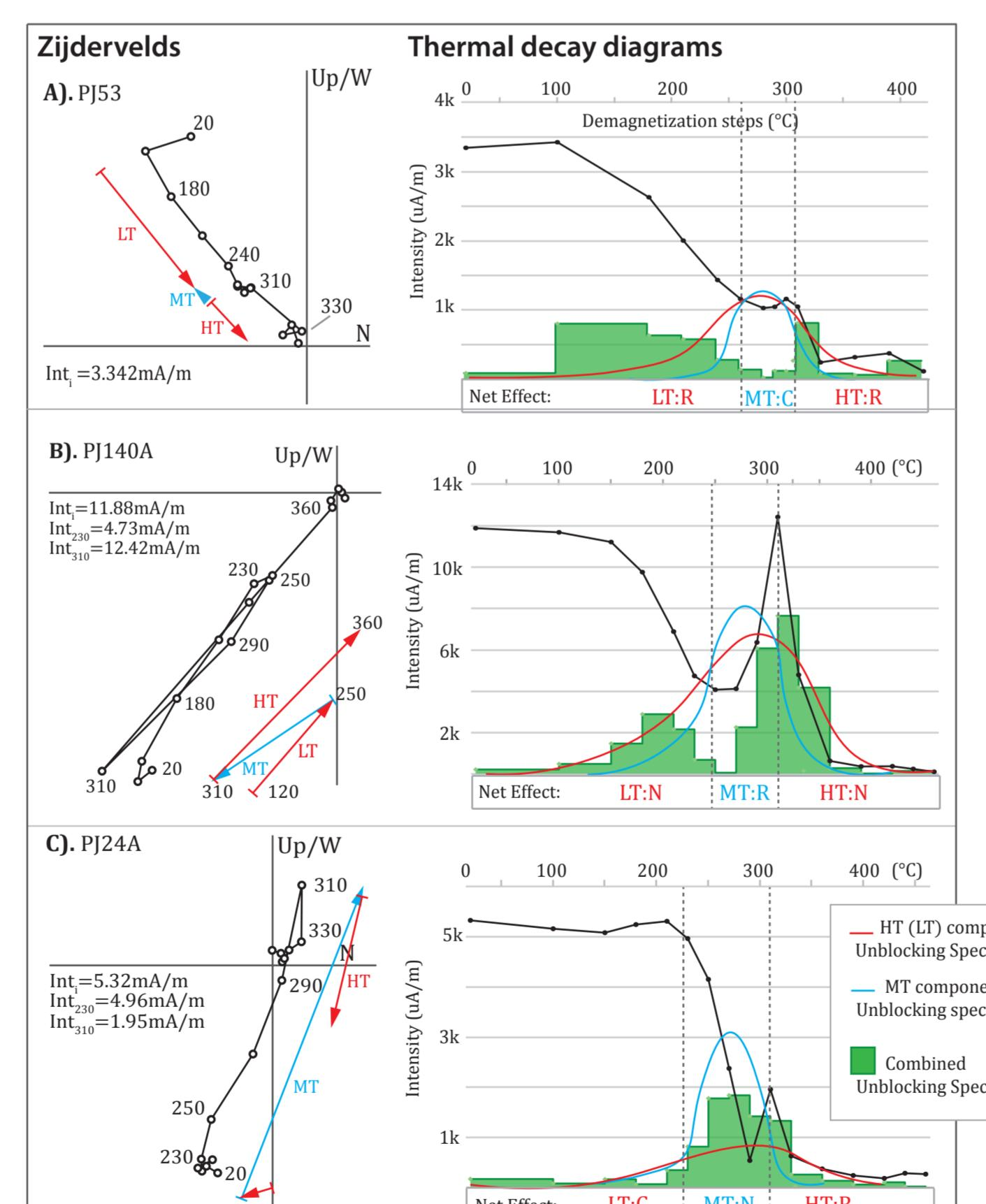
Zijderveld diagrams of M-type samples with varying MT:HT intensity ratios (left) with their corresponding sketched unblocking spectra (right). The individual unblocking spectra for the MT (blue) and LT/HT (red) components contribute to the total unblocking spectrum (green), and explain the variation in NRM behavior in the Zijdervelds.
