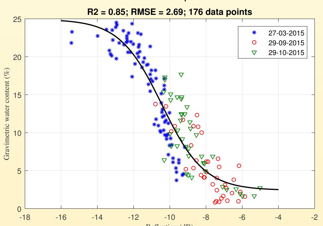
Calibration curve of reflection versus gravimetric surface moisture content. The curve has a range of 2% until 25% soil moisture with a corresponding range of -4 dB to -16 dB, respectively. The calibration curve consists of 176 data points with a RMSE of 2.69% and an R-square of 0.85
