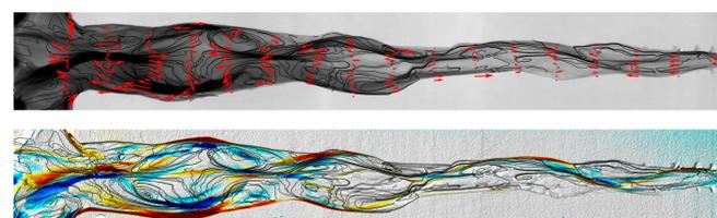
Fig. 10: (top) Streamlines and residual currents after 4400 cycles based on surface PIV, on top of a Digital Elevation Model. (bottom) Digital Elevation Model of Difference (DoD) for period between 4400 and 6900 cycles with streamlines.
