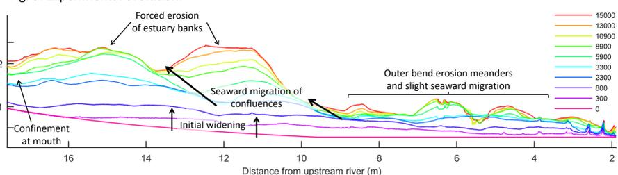
Fig. 6: Evolution of width profiles in the experiment.
