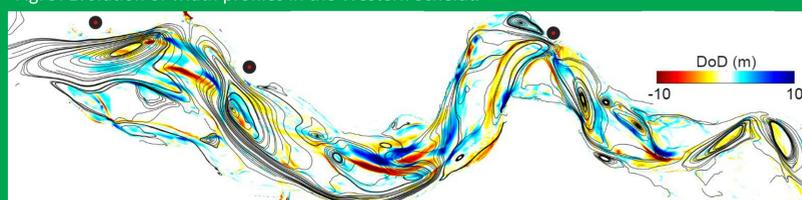
Fig. 11: Streamlines on top of a Digital Elevation Model of Difference (DoD) for Western Scheldt. DoD is based on the difference in bathymetry between 2009 and 2015, streamlines are given for the SCAL-WEST model (RWS) on bathymetry of 2009.
