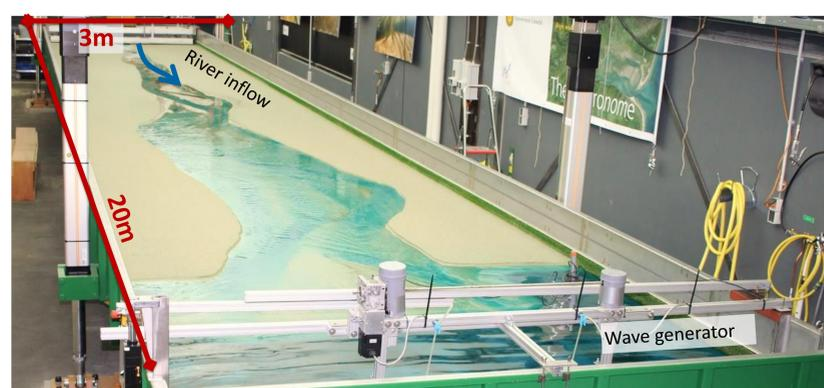
Fig. 4: Overview of the Metronome. See for more details Kleinhans et al. (2017) submitted to E-Surf.
