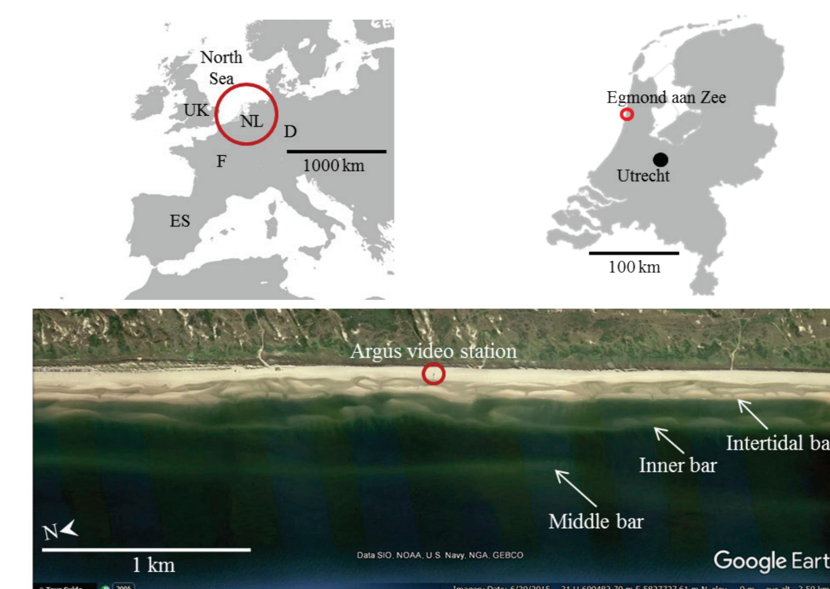
Figure 2 Location of the field site. This wave-dominated, microtidal straight stretch of coast contains three subtidal bars and an ~50-m wide beach backed by a dune system. The bars exhibit net offshore migration over a period of ~15 years, before decaying ~700m offshore.
