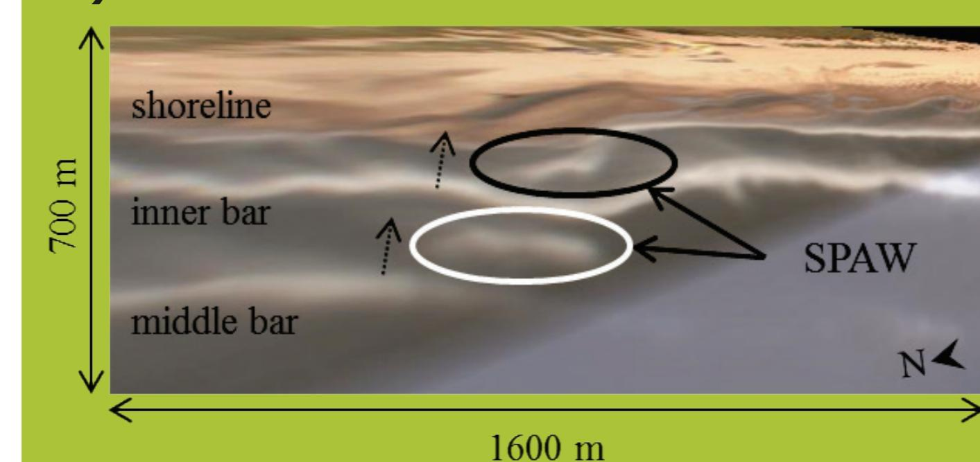
Figure 1 SPAWs, as seen in a time-exposure planview image of the surf zone.
