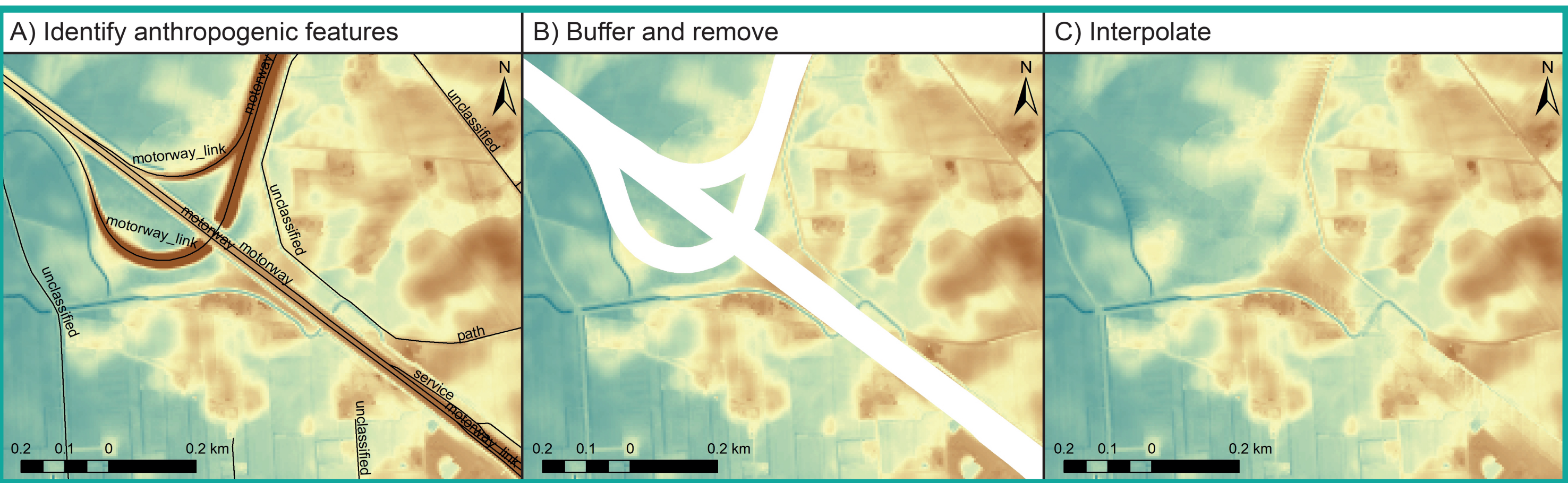
Fig. 3. Automated removal of highway taluds from DEM using OpenStreetMap vector data.
