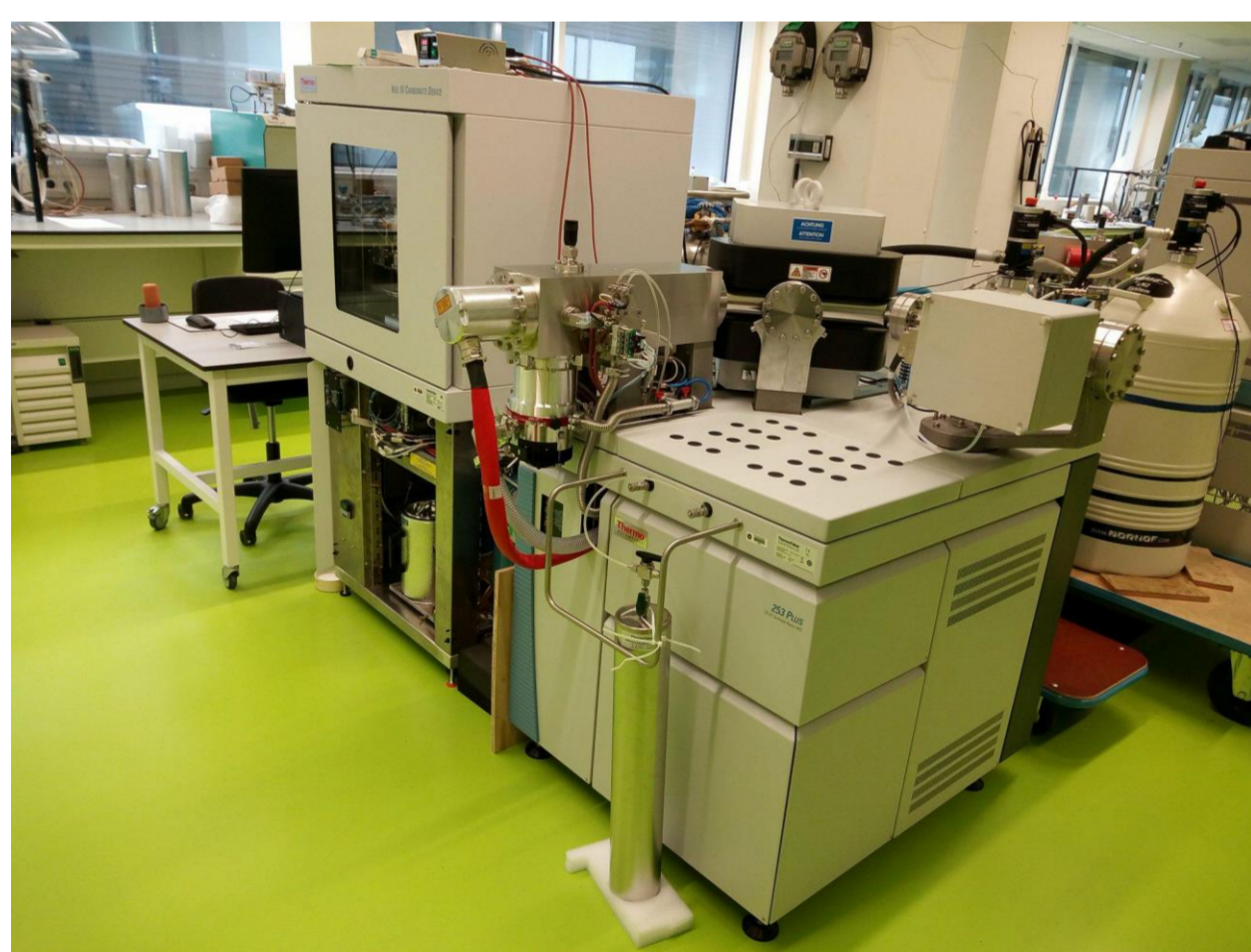
Kiel IV carbonate device (70-95 µg replicates), 102 % phosphoric acid 70 °C, porapak Q trap held at -40 °C, connected to 253 Plus (Thermo Fisher Scientific).
