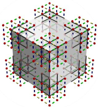
Figure 1 Staggered spatial discretization in 3D.
