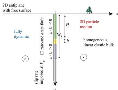
Figure 2 The benchmark problem model setup. (After [2])
