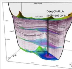
Figure 2: A 3D representation of Lake Chala's sedimentary infill, also showing the coring location (Moernaut et al., 2010).
