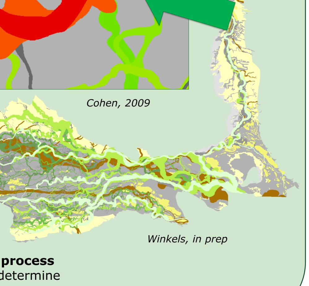
toplayer occurs, creating a **concentrated** seepage outflow point. Since such potential locations are fixed this predetermines the associated discharge and potential for piping to occur. Potential upburst and piping locations are thus fixed to the **position of channel belts** as they determine **regional flow paths**.
