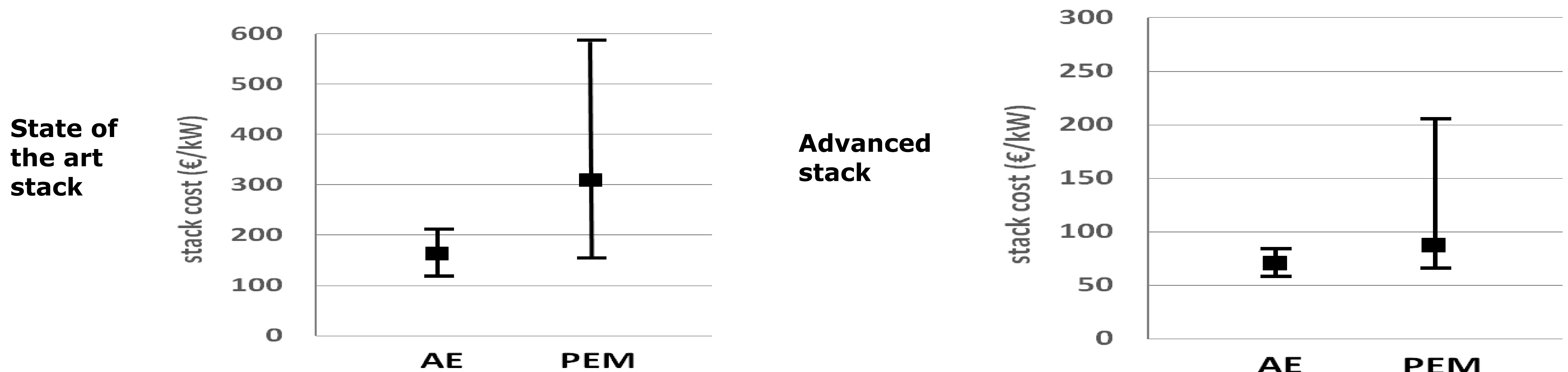
Figure 3: Total direct stack cost including overhead and profit margin a) State of the art stacks; b) Advanced stacks
