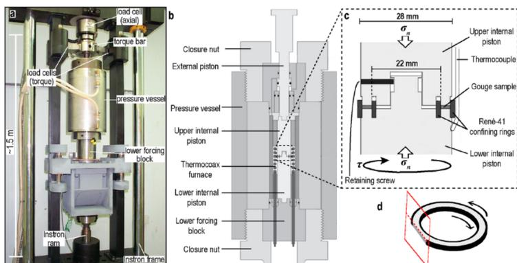
Figure 4: Picture of the unique hydrothermal rotary shear apparatus at the HPT Laboratory (a) and diagrams showing the configuration of the pressure vessel (b), sample assembly (c) and sample configuration (d). From Verberne et al (2015).
