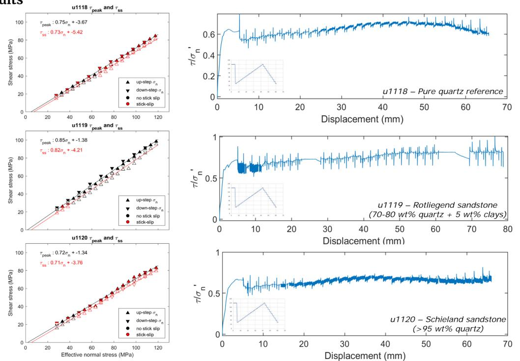
Figure 5: Shear stress vs. effective normal stress plots of the peak (after 1000 seconds hold) and steady state shear stress with linear fits. Slopes indicate the friction; intercepts give the cohesion. Data are derived from the run plots on the right-hand side.
