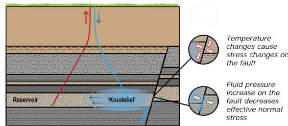
Figure 1: Diagram illustrating the principle of geothermal energy production and two mechanisms to potentially reactivate pre-existing faults
