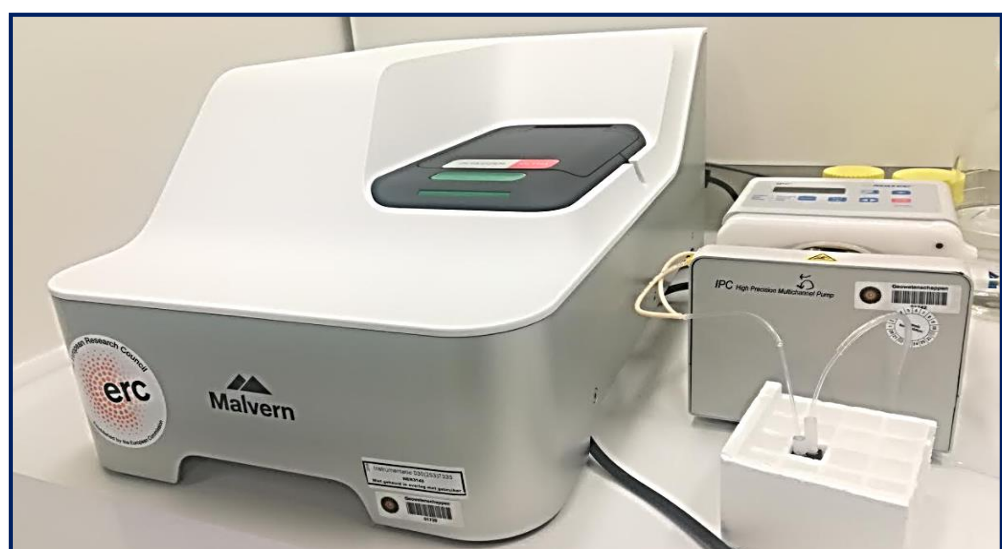
Fig. 2: Experimental set up, Malvern Zetasizer
