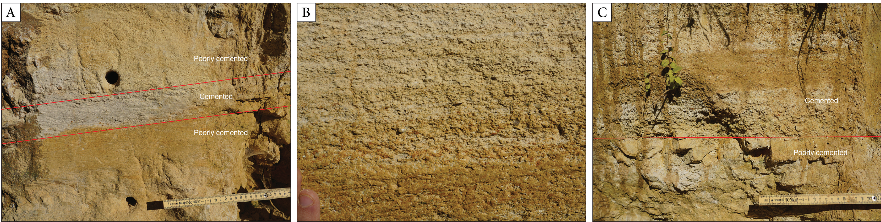
Figure 6 | A Lower part of the Kunrade quarry. Alternation between poorly cemented brownish-orange very fine-grained bioclast-bearing calcarenite and cemented brown fine-grained bioclastic-bearing calcarenite. B Cemented brown fine-grained bioclast-bearing calcarenite. C Upper part of the Kunrade quarry. Contact between poorly cemented brownish-orange fine-grained bioclast-bearing calcarenite and cemented brown fine-grained bioclast-bearing calcarenite.
