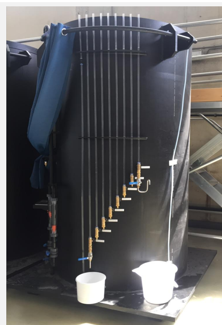
Figure 2: Pilot scale filters which represent real scale slow sand filters
