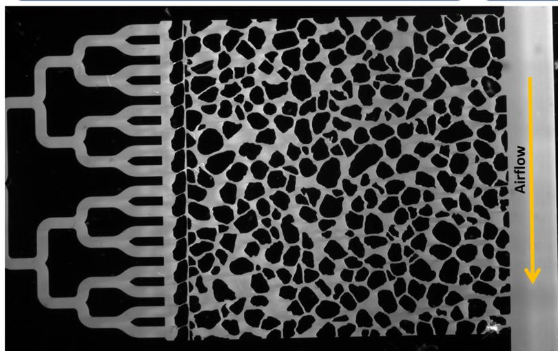
Fig. 1: Design of the microfluidic. Dimensions: 1 cm long & 1 cm wide (magnification of 7x).
