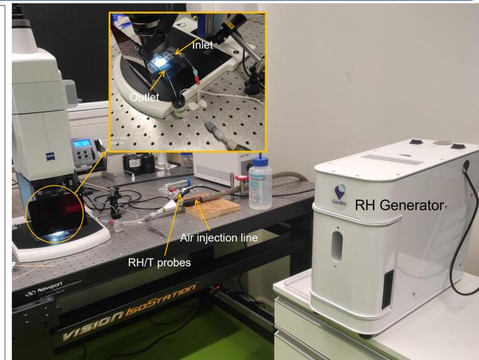
Fig. 3: Microfluidic experiment setup.
