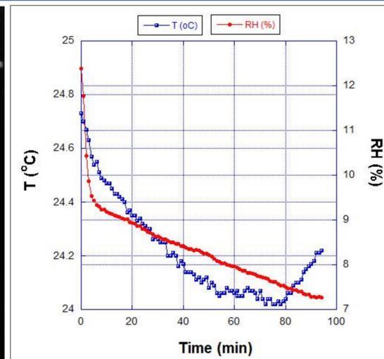
Fig. 2: Variation of relative humidity (RH) of injected air and temperature (T) over time.
