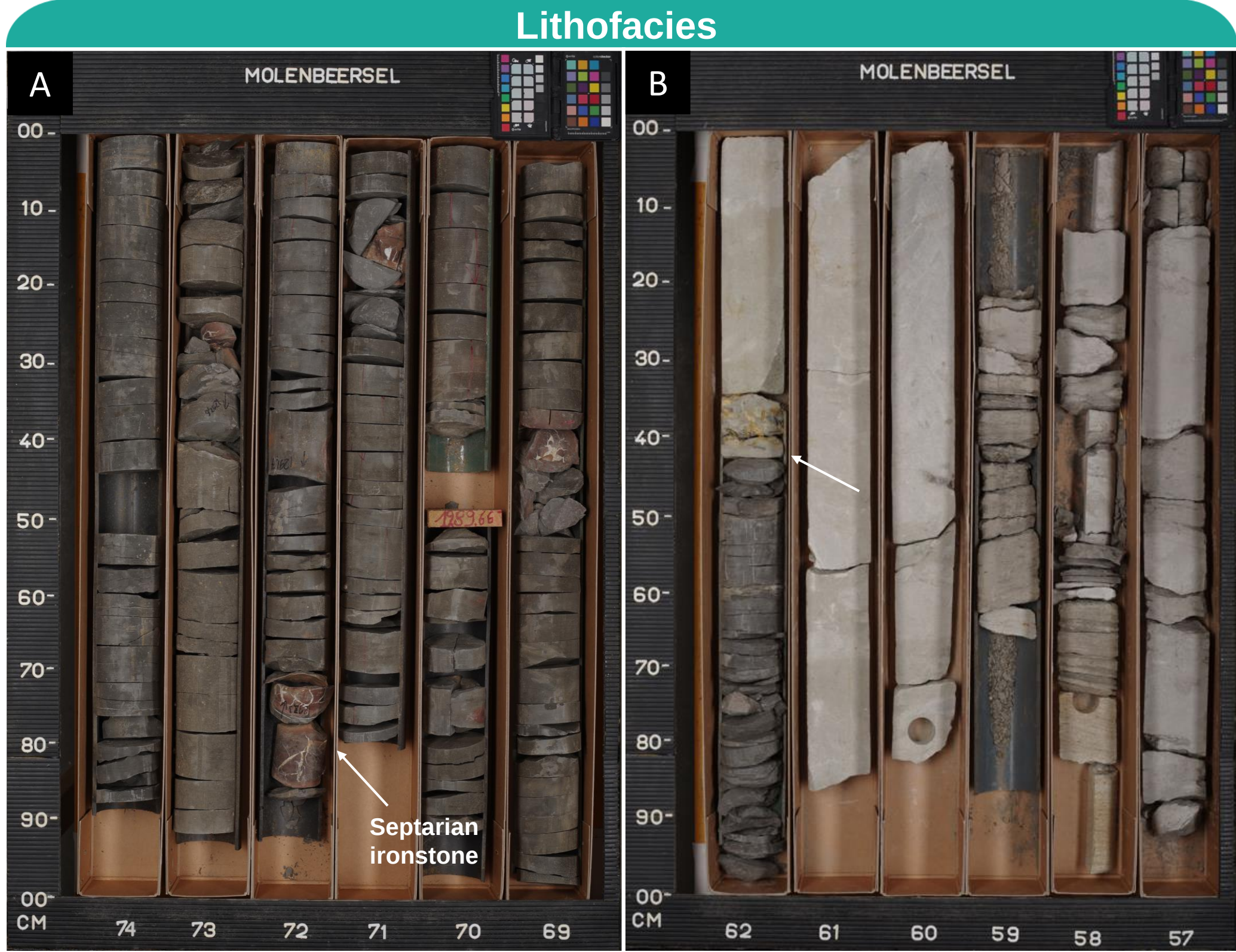
Figure 5 | Aalburg Formation in the Molenbeersel borehole. A) Example of the mudstones with ironstones in the upper part of the core. Sometimes the ironstones present septarian carbonate veins (white arrow). (1288.72 – 1293.94 mbsf) B) Contact between the Lower Jurassic and the Cretaceous deposits (white arrow) (1283.15 mbsf).
