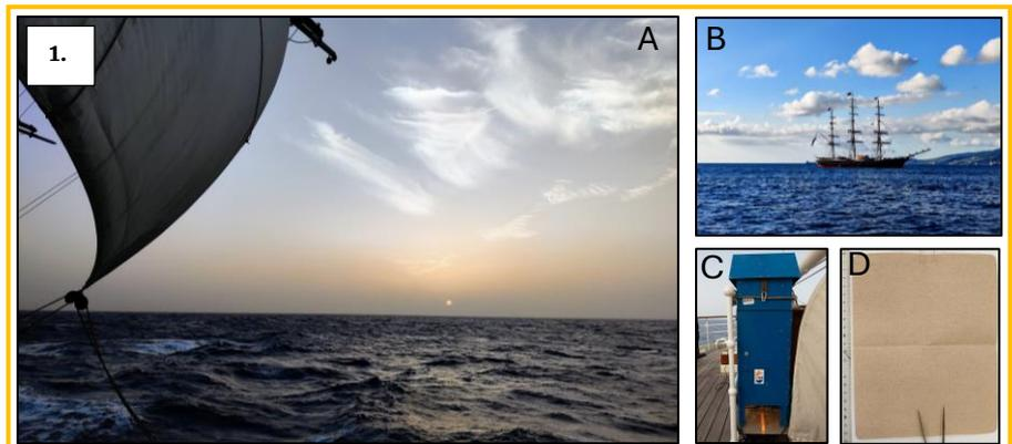
Figure 1 (A): An example of how dust reduces visibility over the North Atlantic Ocean (photo taken during sample A4); (B): clipper Stad Amsterdam in the harbour of Martinique; (C): NIOZ dust sampler mounted on the deck of clipper Stad Amsterdam; (D): An example of a cellulose acetate filter after 24h collection time (~1,800 m<sup>3</sup> of filtered air).
