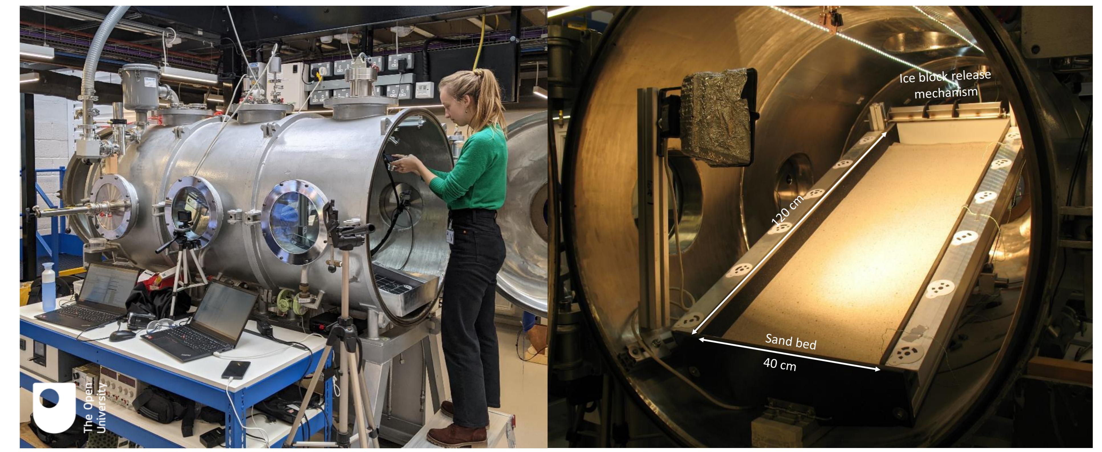
Fig 5 Photos of the experimental set-up. Left, the Mars Chamber (The Open University) from the outside (Lonneke for scale). Right, the flume set-up.
