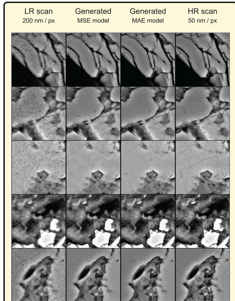
Fig. 2: From left to right: LR tiles that have been resized from 64x64 to 256x256 pixels using bicubic interpolation to match the HR tile size, generated data using a model that was trained using MSE (50 epochs) and MAE (150 epochs) loss functions, respectively, and the corresponding HR tiles.
