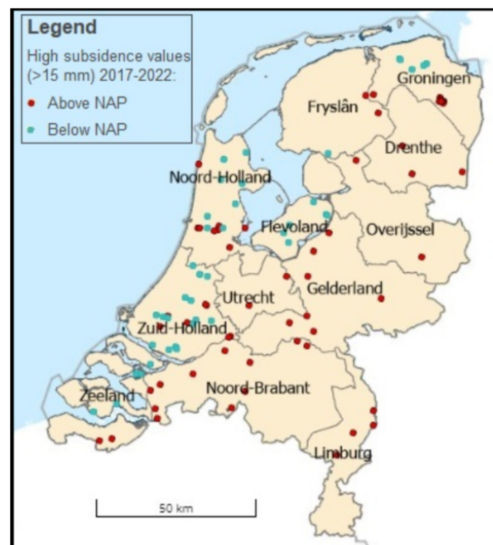
An analysis of remote sensing land subsidence data between 2017-2022 (Hammad et al. 2024)
